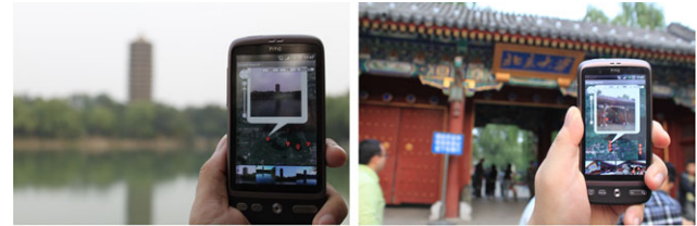
Fig. 7 User interface of our mobile landmark search, which is developed in HTC DESIRE G7 smart phone (512 MB ROM + 576 MB RAM memory, an 8G extended storage, a 528 MHz processor, and an embedded camera with maximal 2592 \times 1944 resolution)
