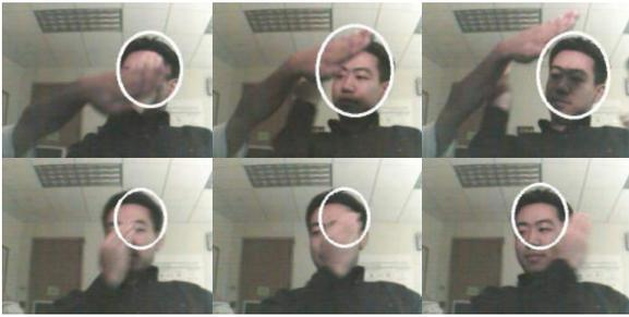
**Figure 11. Tracking with partial occlusions**
