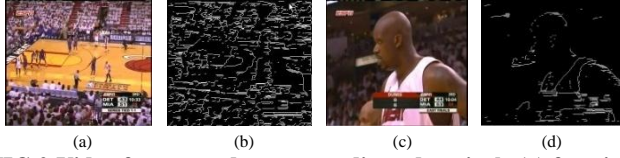
FIG.2 Video frames and corresponding edge pixels (a) far-view frame (b) edge pixels of far-view frame (c) close-up frame (d) edge pixels of close-up frame
