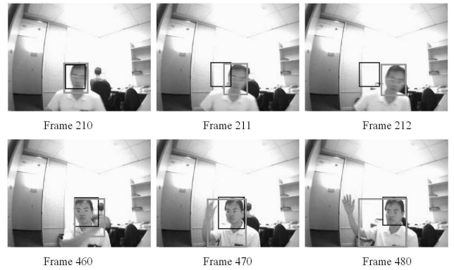
Fig. 4. Test of different proposal modules: On the first row, the contour tracker (black bounding box) loses track when the person suddenly moves but the color tracker (blue bounding box) survives. On the second row, the color tracker module fails when the person's arm waves in front of the face, but the contour tracker succeeds.
