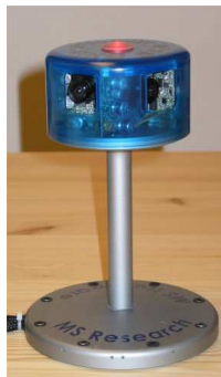
Figure 5. RingCam: an inexpensive omnidirectional camera and microphone array designed for capturing meetings.
