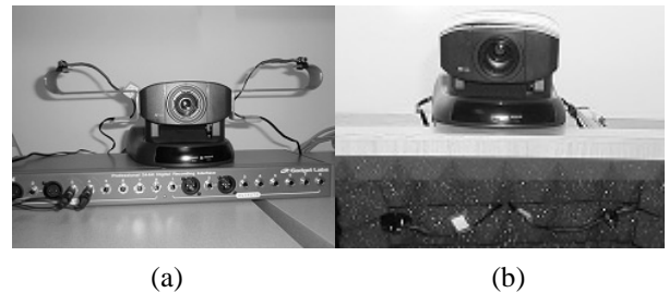
Figure 6. (a) Microphones are attached to extension structures of the active camera; (b) Microphones (lower portion of the figure) are separated from the active camera.
