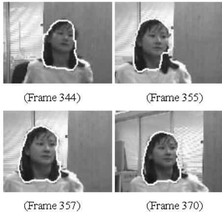
Fig. 3. Tracking with our new contour model. The tracking results quickly recovered when the user moves away from the door.
