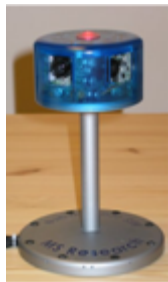
Figure 1: RingCam: an inexpensive omni-directional camera and microphone array designed for capturing meetings.
