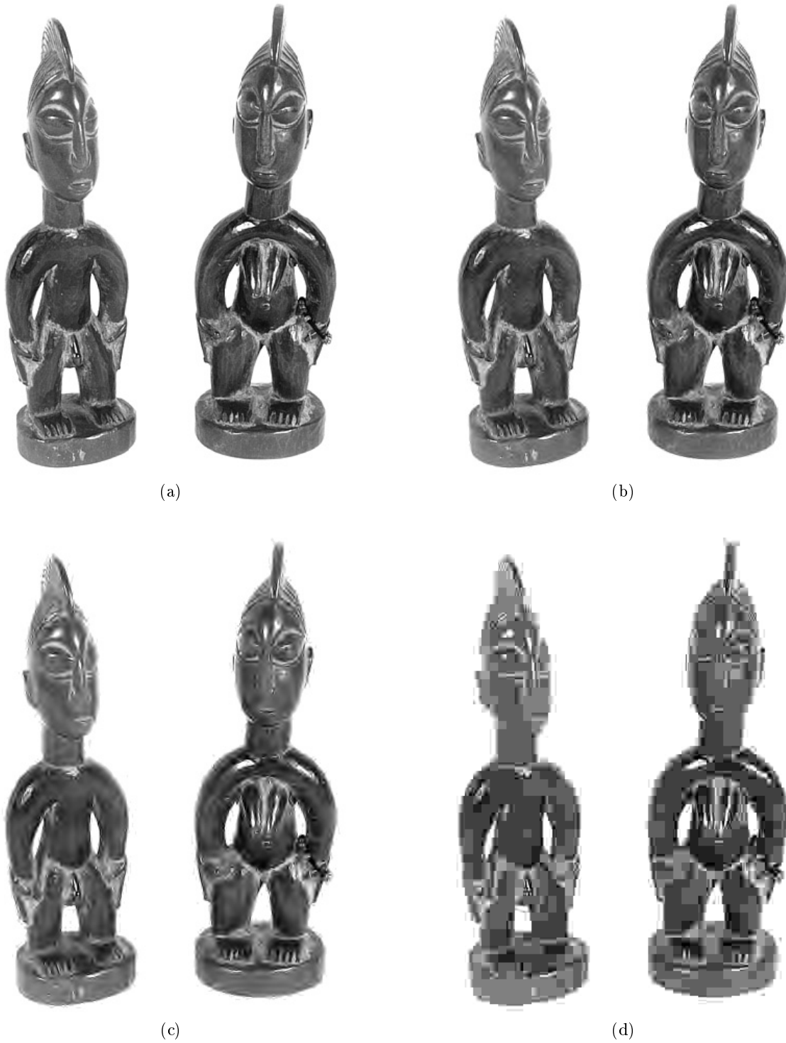
Fig. 6. Sample reconstructions of the still image coder, case 2: (a) the original image (1306624 bits, 8bpp), compressed by factors of (b) 16:1 (81664 bits, 0.5bpp), and (c) 47:1 (27766 bits, 0.17bpp). For a perceptual quality comparison, (d) shows a JPEG reconstructed image at 0.17bpp.
