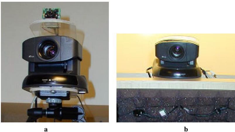
Fig. 4. a Lecturer-tracking camera: the top portion is a static wide-angle camera. b Audience-tracking camera: the lower portion is a two-microphone array used to estimate sound source location
